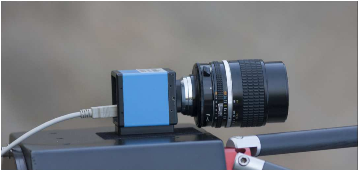
Fig. 11 Camera and 100 mm focal lens on piggy-back of the same 10" RC telescope from previous picture
