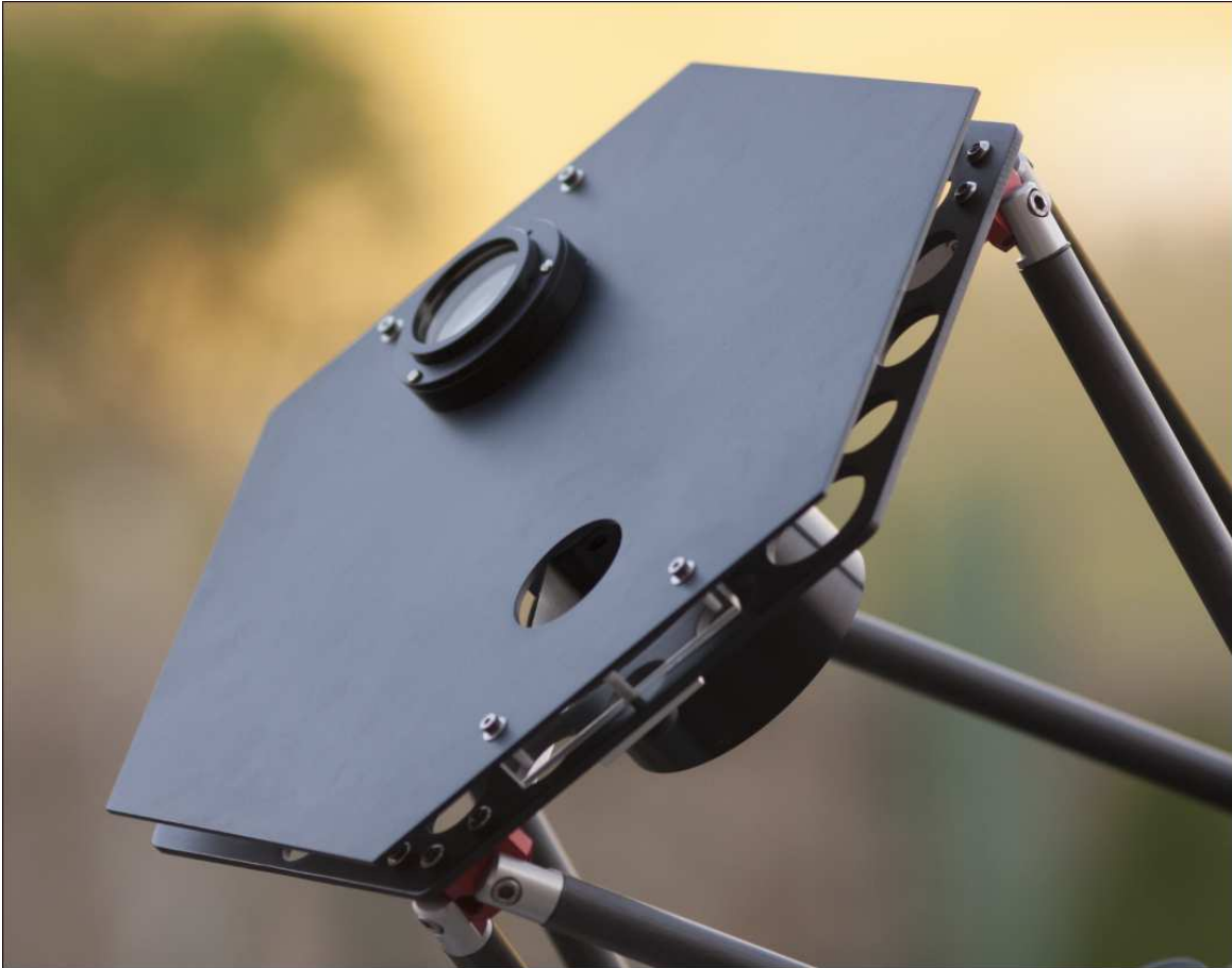
Fig. 10 Complete mask on top of a 10'' RC telescope
