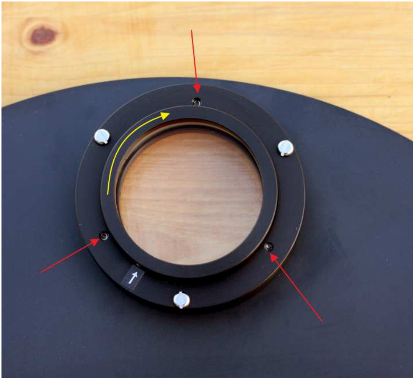
Fig. 8 ALCOR SYSTEM deviation tunable prism : how to adjust beam deflection
