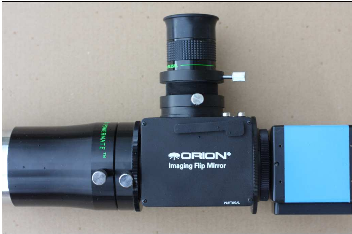
Fig. 14 Flip mirror and eyepiece for field centering
